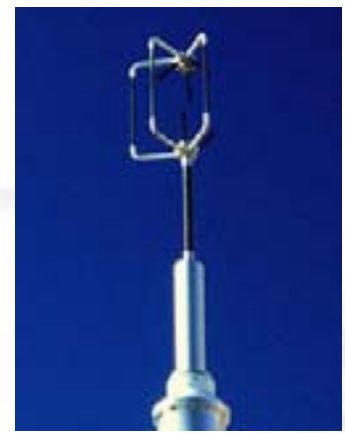
Sonic anemometer (4.5 meter) : three wind components measurements; used for SR calibration
