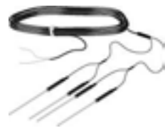
Soil temperature thermocouples (buried at a depth of 4-1 cm)
